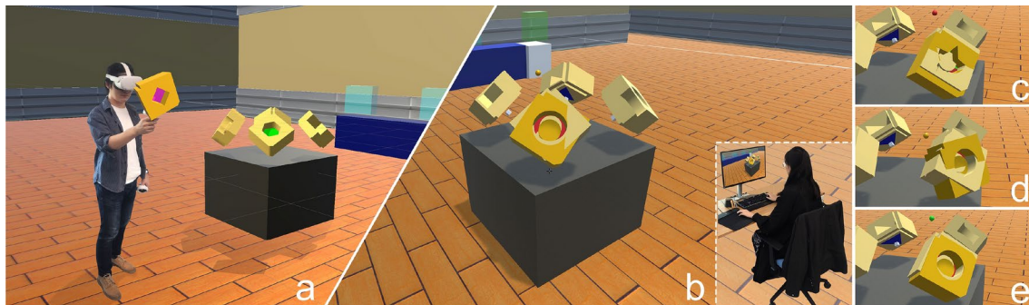
Fig. 3 Figures showing the manipulation methods when using a VR controllers and b PC mouse and keyboard. c An incorrect target object with the red sign; d a correct but not aligned object with the orange sign; e a correct and aligned object with the green sign
